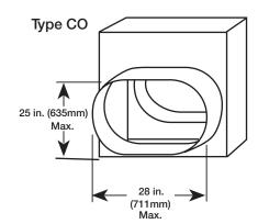
C, CO, CR transitions are positioned 1 in.(25mm) from bottom of sleeve.
